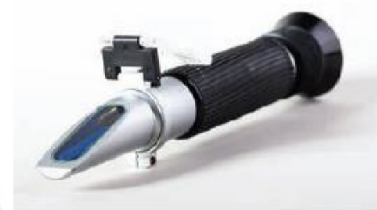
Figure 4.3 Refractometer for measuring the ripeness of grapes. The same method is used by optometrists to measure the refractivity of a patient's eyes
