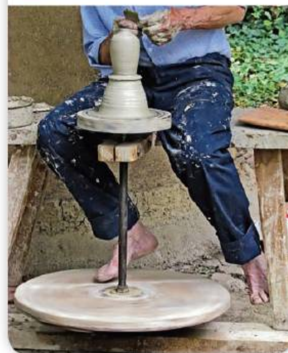
Figure 11.4 A potter's wheel takes a lot of force to spin around, but then keeps spinning
